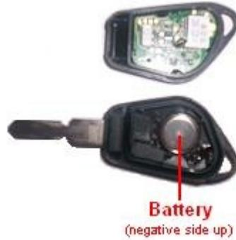
Note the position of the batteries (negative side up), replace with two CR 1620 3volt batteries.
